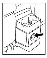
Turn the wing nut on the cover counterclockwise to remove it.
